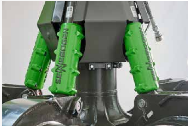
Solid protection for cylinder rod
