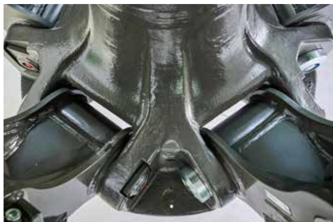
Openings at the shell pivot points for low-maintenance operation
