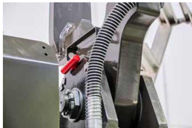
Pin mounting for vertical fixing of the grab mount
